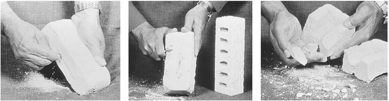
Figure 3-31 Under-burned bricks are easily scratched or scored with a coin, cut with a knife, or broken by hand. (Photos courtesy Brick Institute of Texas.)
